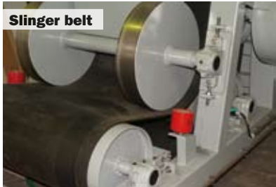
Application: slings bulk material in the corners of cargo hold
